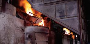
Our specially designed side draft hoods are meant to ensure highly effective and efficient suction of fumes even while feeding scrap through magnet or grab or poking of scrap during melting operations.
